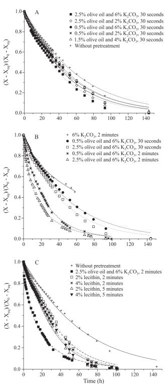
**Figure 2.** Drying curves for Rubi grapes dried at 50°C and air velocity of 1 m s<sup>-1</sup>. Traces represent the adjustment of Page model (equation 1).
