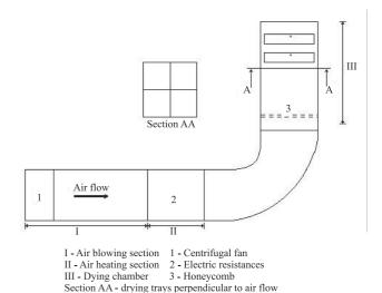
**Figure 1.** Schematic diagram of resistive dryer with crossed airflow.
